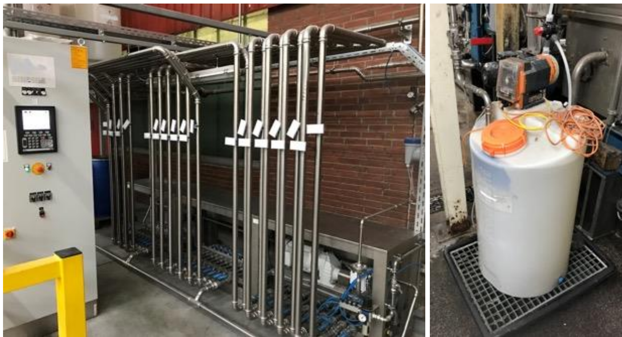
Figure 5: Example of a closed automated dosing (left) and mixing system (right) of a continuous washing machine
