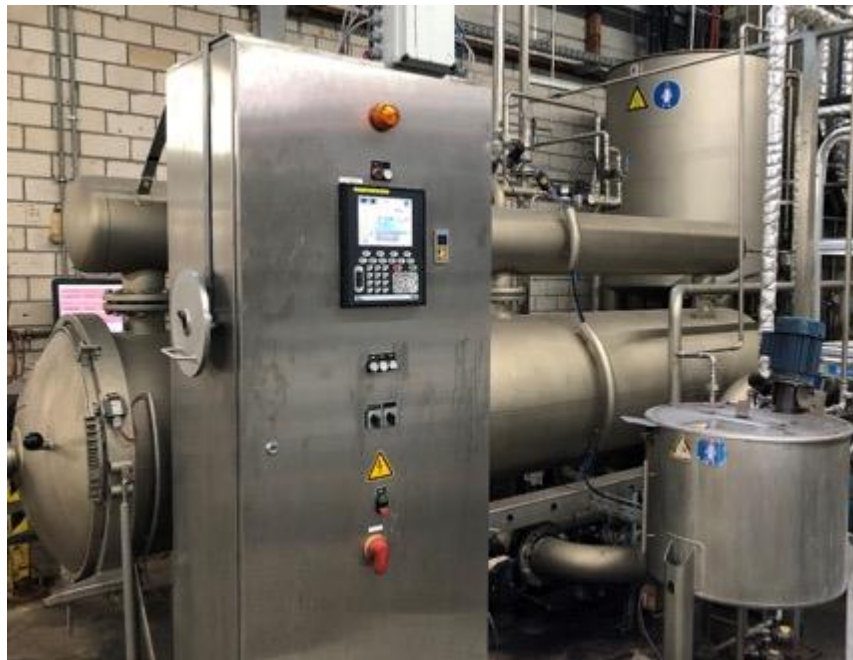
Figure 11: Example of a dyeing machine used to treat textiles. In the lower right corner, the automated dosing and mixing system can be seen.
