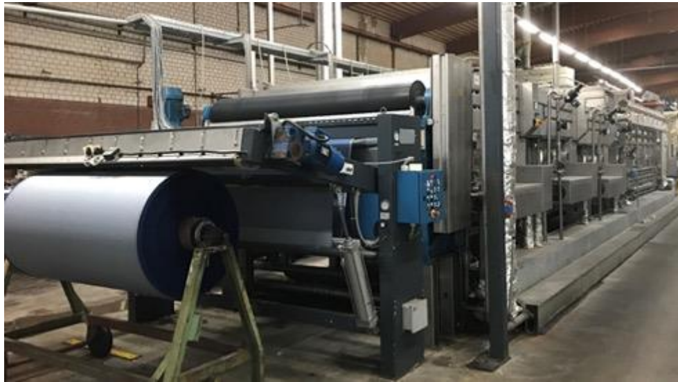
Figure 7: Example of a continuous washing machine
