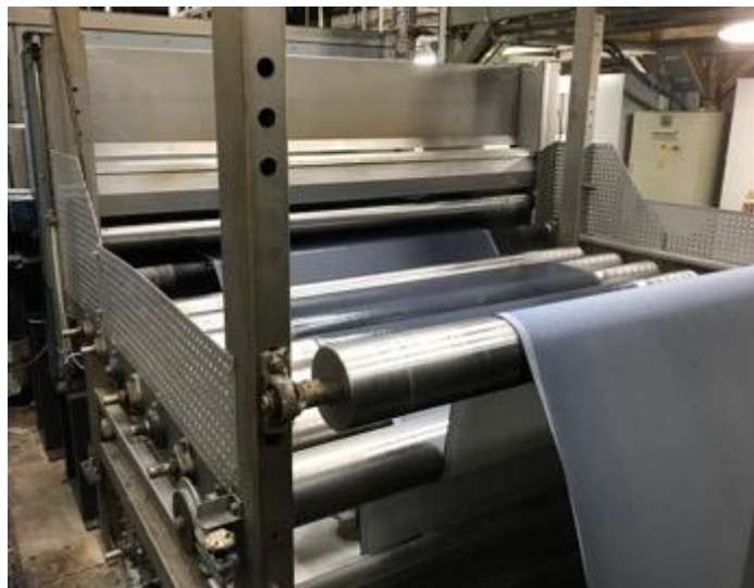
Figure 10: First processing step (typically de-sizing) of a continuous washing machine
