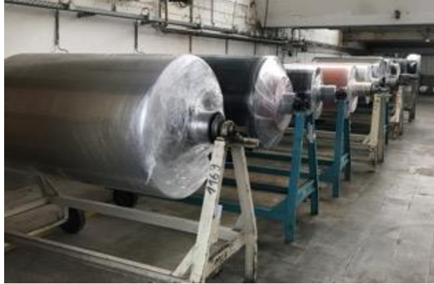
Figure 8: Example of a cold pad-batch treatment
