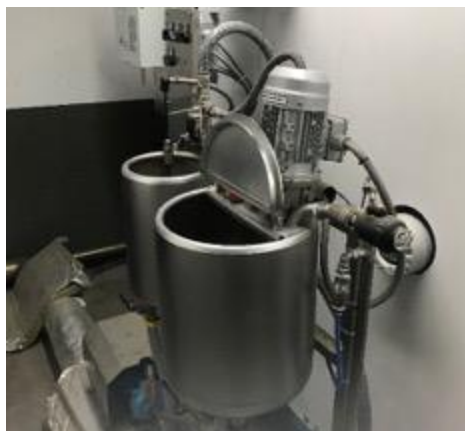
Figure 14: Mixing tank on the back of a washing machine used in the garment finishing industry
