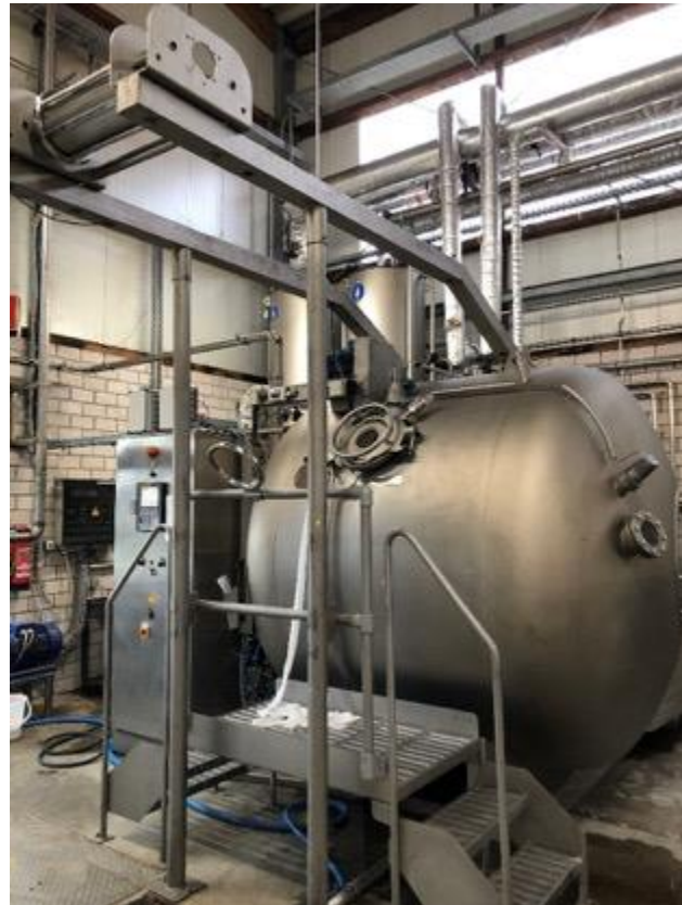
Figure 9: Example of a dyeing machine that is used for batch processes
