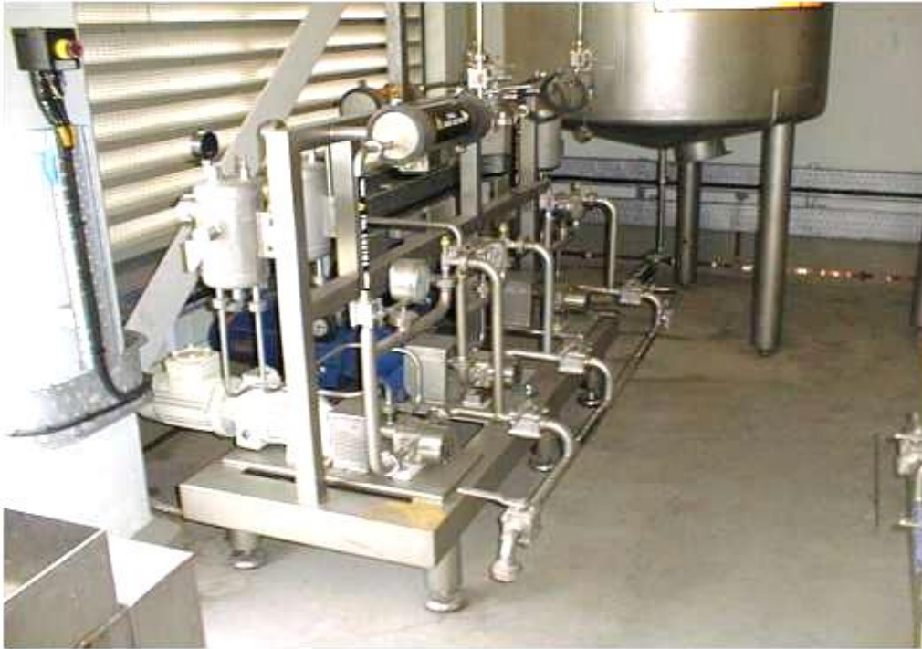
Figure: Example of Enzyme Transfer Pump Sets (source: AISE: Guidelines for the Safe Handling of Enzymes in the Detergent Manufacturing)
