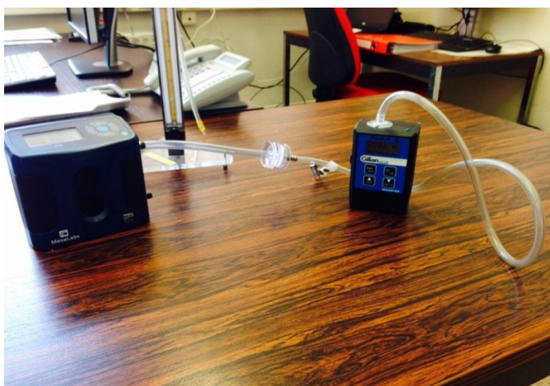
Figure: Calibration set-up for air sampling equipment. ( Courtesy: DuPont Nutrition and Biosciences )
